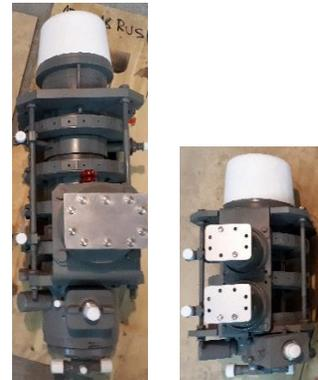
Figure 1: S-band (left) KIU-168 and C-band KIU-271 klystrons [2].
