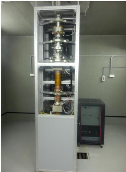
Figure 5: Accelerators for sterilization.
